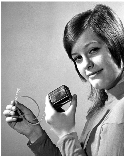
Model of a nuclear-powered heart pacemaker developed by Arco Medical.
